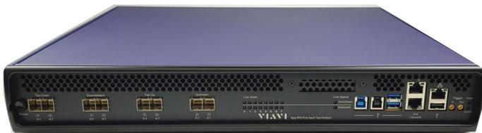
The Xgig® 5P8 platform provides protocol analysis for PCIe 5th generation traffic at all layers of the stack. It supports link widths up-to 8-lanes, and link speeds to 32 GT/s.
