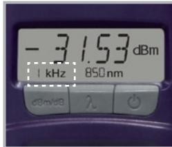
The power meter detects light signals modulated at standard frequencies of 270Hz, 330Hz, 1kHz, and 2kHz. If one of these frequencies is detected, it appears in the display. At very low input levels, the modulation signal cannot be identified, in which case 2 hyphens "--" will appear.
