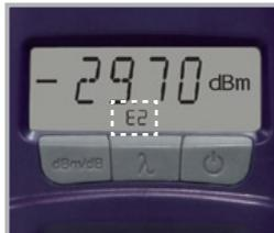
When first powered on, the power meter runs a self-test that checks the program and calibration data memory. If an error is detected, an error message is displayed at the end of the self-test.
