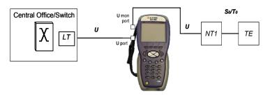
Figure 8 Connecting as a U Monitor
