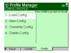
**Storing test** After you finish specifying the HST-3000 for a particular test. profiles you can store the test profile for future use. You can store up to 10 profiles.
