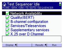
The check mark indicates that the test will be included in the test sequence.
