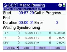
The test will run for the duration set in the BERT configuration menu.
