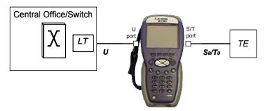
Figure 7 Connecting as a NT1 Replacement
