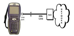
If connecting behind a full-rate splitter, use a cable that will connect the VDSL signal on pins 2 and 5 to pins 4 and 5 on the HST-3000 as shown below.
