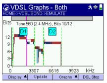
The dotted line separates the band plans, indicating the upstream (U) and downstream (D) frequencies. If they do not appear, press the **Graphs** soft key and then **Show Band Labels**.
