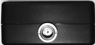
This connector is for RF signal input. It is an "F"-type male connector.
