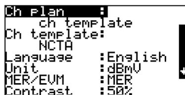
To change active Channel Plans or to change the Channel Template within the MSQ-900, go to the Setup menu and use the up ▲ and down ▼ arrows to select the Configuration setting
