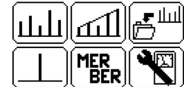
To select the desired function in the main menu, press the up ▲ or down ▼ arrow key to move the corresponding icon to the bottom line of the screen. Then press the Function key which is under the required icon. Press the EXIT key to return to the main menu.
