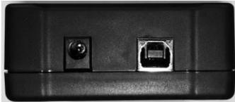
The Power (DC 12V) connector is for connection to an external power source (charger) and the USB connector is for connection to a computer.
