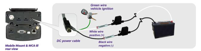
\*Use the provided in-line fuse holders to wire the white & black DC power cables to the vehicle battery as shown. Wire the green DC power cable to the vehicle key switch to allow the MCA III to determine when the vehicle is turned OFF.
