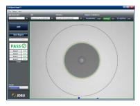
Press the QuickCapture button on the probe OR click the TEST button from the FiberChekPRO toolbar to run analysis.
