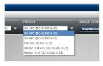
From the pre-configured PROFILE settings dropdown list, select the appropriate connector being inspected.
