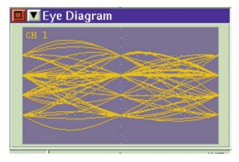
Figure 4.0 - The P25 Eye Diagram
