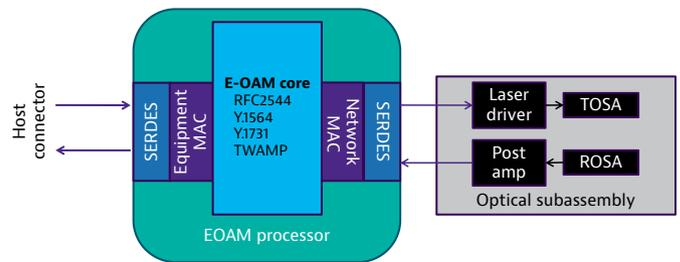
Figure 1. Simplified optical block diagram of JMEP3
