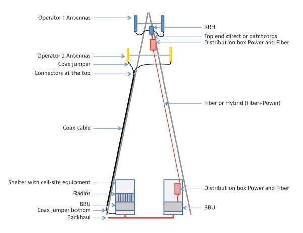
Figure 5: Common cell site structure and components
