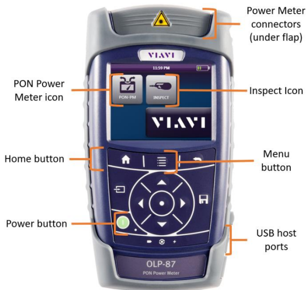
Figure 4: OLP-87, Front View
