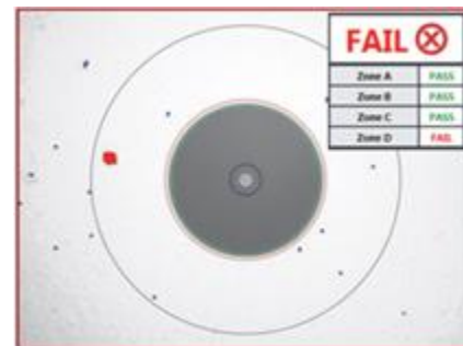
Figure 3: Image of Dirty Fiber
