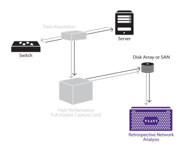
Architecture of a typical Retrospective Network Analyzer
