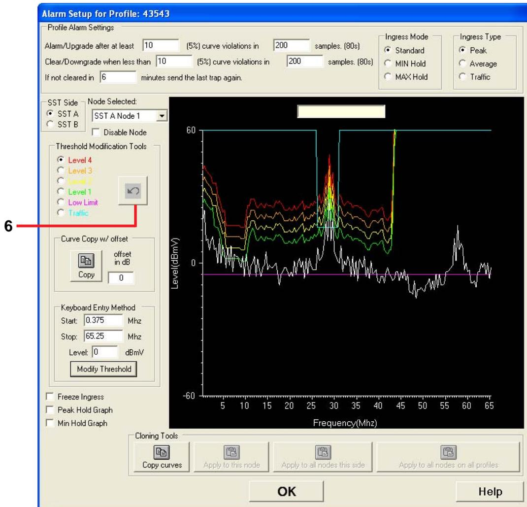
1. The **Profile Alarm Settings** heading will automatically be filled in by the instrument. Modify the values if needed.
