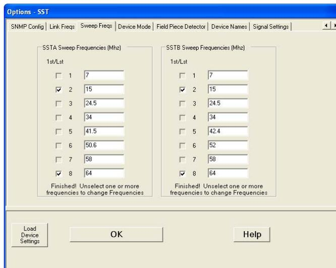
2. On this tab the sweep frequencies used in conjunction with the telemetry to the field pieces will be entered.
