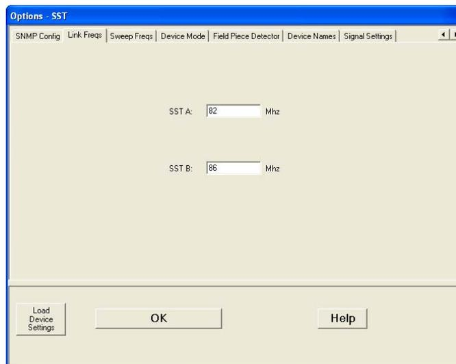
2. On this tab the link frequencies to be used in sending telemetry to the field pieces will be entered.
