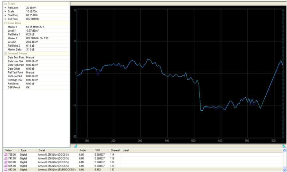
The Scan Data View Graph compares the levels at two different points in the cable system. In this view, the light blue line is a plot of the measured scan of all channels. The dark blue line is a reference scan that was previously taken at a different place on the cable network and stored for reference purposes.
