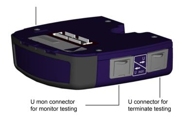
Figure 6 BRI interface connectors
