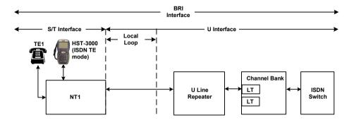
Figure 3 ISDN TE mode for the S/T Interface
