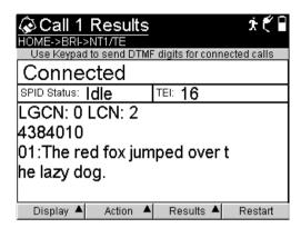
If you transmitted the FOX text to another test device, verify that the correct text was received on the far end.
