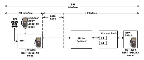
Figure 5 HST emulation modes for BER testing the BRI Interface
