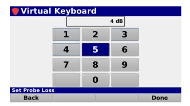
When finished entering the test point loss information, press the **Back** button to return to the **Channel Plan Scan** screen.
