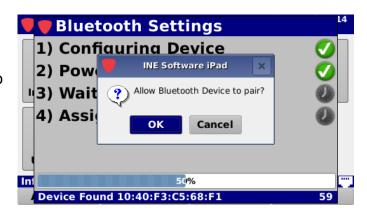
Once the 720 DSP connects to the iPad, the **Bluetooth Settings** window will display the network connection progress.
