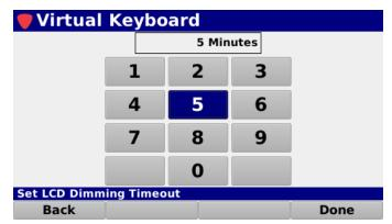
Upon any button press, the LCD will automatically brighten and the delay timer will restart.
