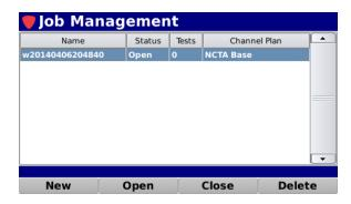
By default, the **Channel Plan** field will be populated with the last used channel plan provided that it still exists on the instrument.
