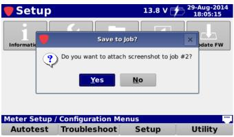
If you don't want to save the test to the open job, select **No** and you will be prompted to enter a file name using the **Virtual Keyboard**. It will then be saved to the internal memory of the 720 DSP.
