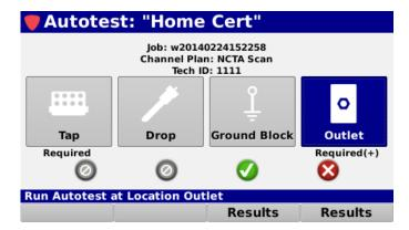
Location Pass/Fail Indicators – Each location will display a pass/fail indicator as shown in the following section:
