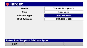
Once you have selected the Address Type, select the MAC Address, Host Name or IPv4 Address field and use the Virtual Keyboard to enter the address of the target loopback device as shown in the images below.
