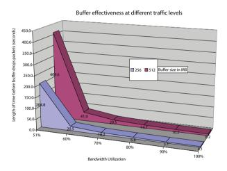
**Please Note:** The role of the buffer is to absorb traffic spikes of over 50% full-duplex bandwidth saturation, because the analyzer's single-receive interface simply cannot move the bits fast enough to keep up at line rate. The data in the buffer is released when utilization drops to the point where the analysis interface can move both the "live" data plus the data released from the buffer. Packet loss is unavoidable if the utilization spikes exceed the capacity of the buffer.
