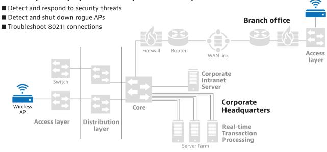
With probes and TAPs deployed in such a manner, Widgetco's administrators can see all network traffic wherever they need to, and they can do so from any analyzer console on the network.
