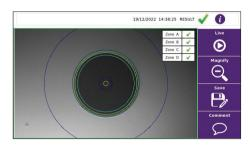
Integrated fiber end-faces inspection with pass/fail analysis
