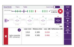
Smart Link Mapper view, simplified icon based view of OTDR test results
