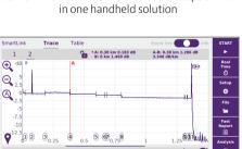
OTDR trace view for expert analysis and additional manual measurements
