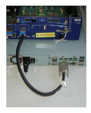
Appropriate Test Setup: 1) Signals are sent over a single cable, 2) the cable is a minimum length (short), and 3) the cable is properly shielded and rated for 6 Gb/s use.
