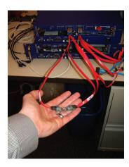
Test Setup to Avoid: Signals are 1) sent over a splice, 2) the extended double cable is longer than required, and 3) the cable used is unshielded.
