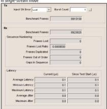
Sequencing: Frame loss / out-of-order / duplicates. Can inject errors on transmit
