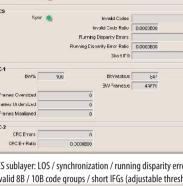
PCS / PMA sublayer: Optical GigE: LOS / PCS synchronization / running disparity errors / invalid 8B / 10B code groups 100BASE-FX: LOS / sync / far end fault / invalid codes MAC sublayer: Frames too long (>jumbo) / jabbers / undersized / fragments / CRC errors / in-range length errors (802.3 frames) / short IFGs (adjustable threshold, does not apply to 10 / 100 / 1000BASF-T)
