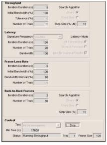
Provides throughput, latency, frame loss, and back-to-back measurements in single stream mode. Up to 10 frame sizes. Supports function to run all tests in succession. Logs results to file and generates graphics
