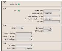
PCS sublayer: LOS / synchronization / running disparity errors / invalid 8B / 10B code groups / short IEGs (adjustable threshold) FC-1: Frames oversized (>2148 bytes) / frames undersized (<36 bytes) / frames misaligned (non-multiple of 4 bytes) FC-2: CRC errors
