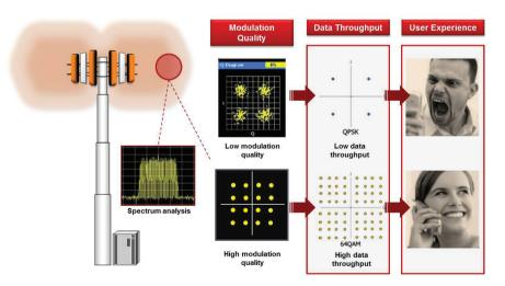
Figure 14. LTE signal analysis; LTE modulation quality indicates the modulation scheme and data throughput assigned to each user
