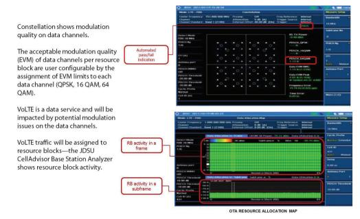
Figure 13. LTE RF signal analysis of VoLTE: demodulation and resource block analysis
