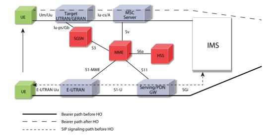
The following diagram illustrates the key network elements and interfaces required to deliver SRVCC.
