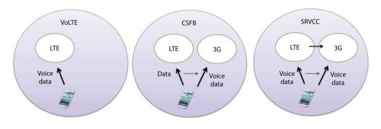
Figure 11. The span of VoLTE, CSFB, and SRVCC
