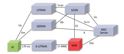
Figure 9. CSFB elements and interfaces (source: 3GPP TS 23.272 V10.14.0)
