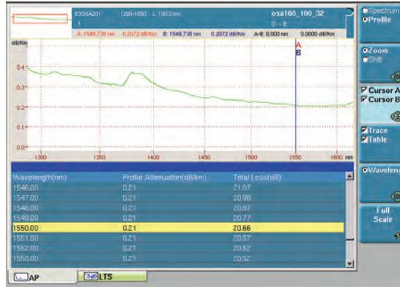
Attenuation Profile measurement with the T-BERD/MTS 8000
