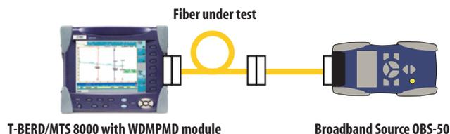
Test setup with JDSU T-BERD/MTS 8000 and handheld broadband source
