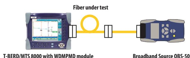
Test setup with JDSU MTS/T-BERD 8000 and full band broadband source module
