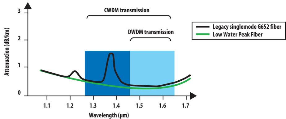
Fiber attenuation as a function of wavelength
