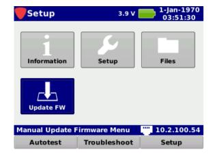
The **Update Firmware** screen will be displayed as shown in the image to the right. This screen allows you to perform a firmware update. Before performing a firmware update, you must accept the End User License Agreement (EULA) by selecting the **Accept** softkey.
