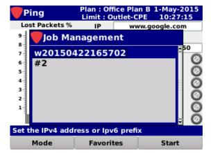
If you don't want to save the test to the open job, select **No** and you will be prompted to enter a file name using the **Virtual Keyboard**. It will then be saved to the internal memory of the 120 DSP.
