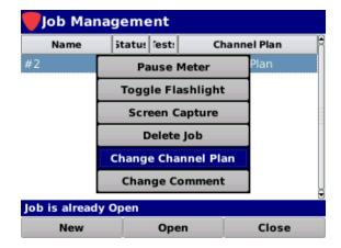
If there is more than one channel plan on the 120 DSP, the **Channel Plan** window will be displayed as shown in the image below (left). Select the name of the channel plan that you would like to assign to the selected job.
