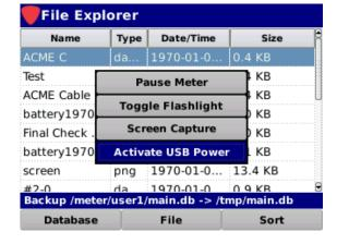
4. The power to the USB flash drive is activated and the drive is now mounted to the file system as shown in the image to the right. The 120 DSP is now capable of transferring files to and from the USB flash drive.
