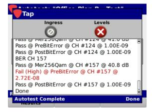
When the Autotest is complete, press the Back button to exit. A notice screen will be displayed as shown in the image to the right. Select the **OK** button to save the test results or select the **Cancel** button to exit without saving the test results.
