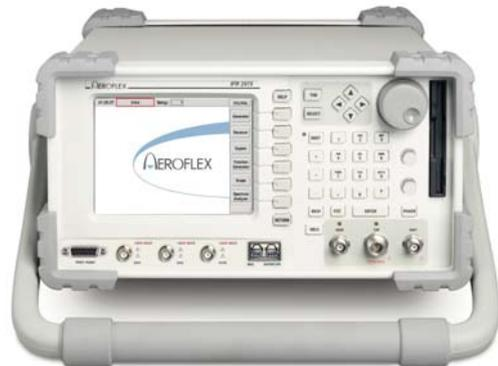
The 2975 P25 and analog radio test set
