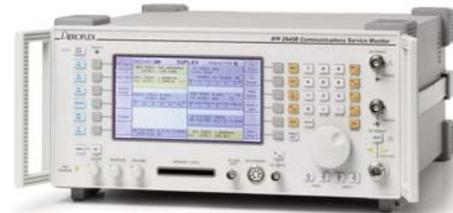
The 2945B Series analog radio test set
