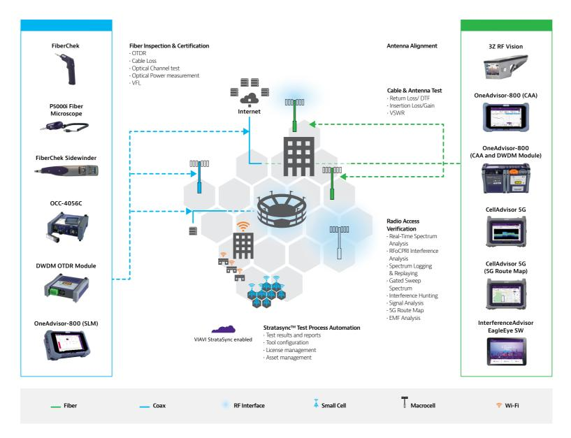
Maintaining 5G in the field can span working on an array of subsystems and situations including layer 1 fiber, cable and antenna system, interference, radio performance, or and radio configuration issues.
