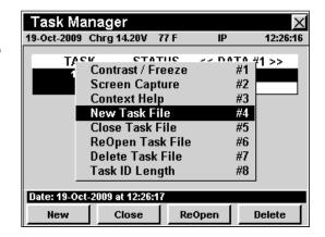
The Function Menu will close and the Create New Task window will open. Use the 1...0 buttons to enter a task ID number, and select the button. The instrument will return to the Task Manager window.
