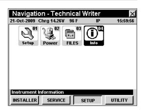
Use the **(A)** v buttons to select the **RF Option Info** field. If the FDR Option is installed, the widow will display the text *FDR*: YES.
