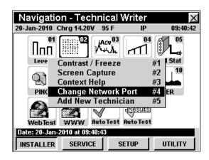
Use the buttons to highlight the **External RJ45**, **Internal Modem**, or **Wi-Fi** network port, and then press the button.
