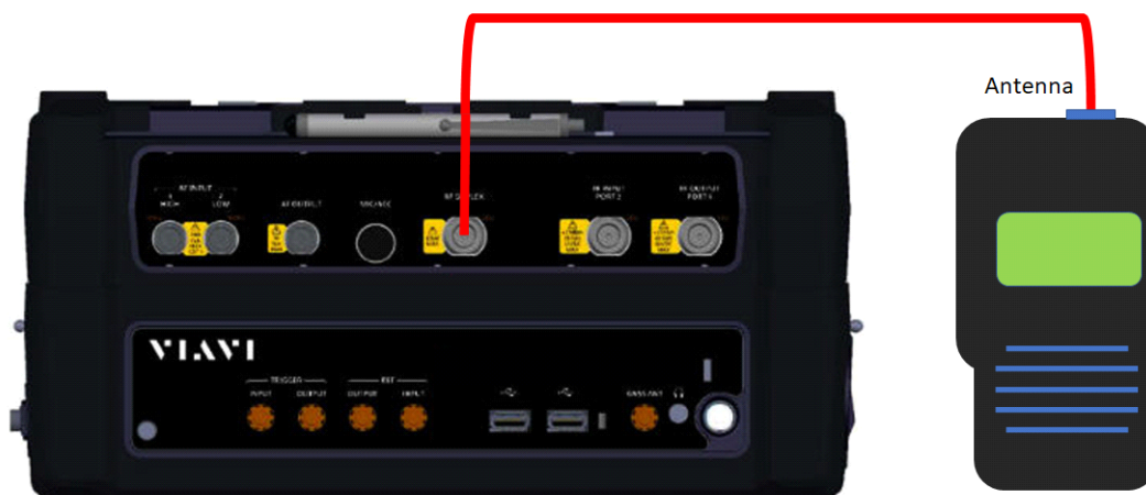
Figure 3-1 P25 Transceiver Test Setup Diagram
