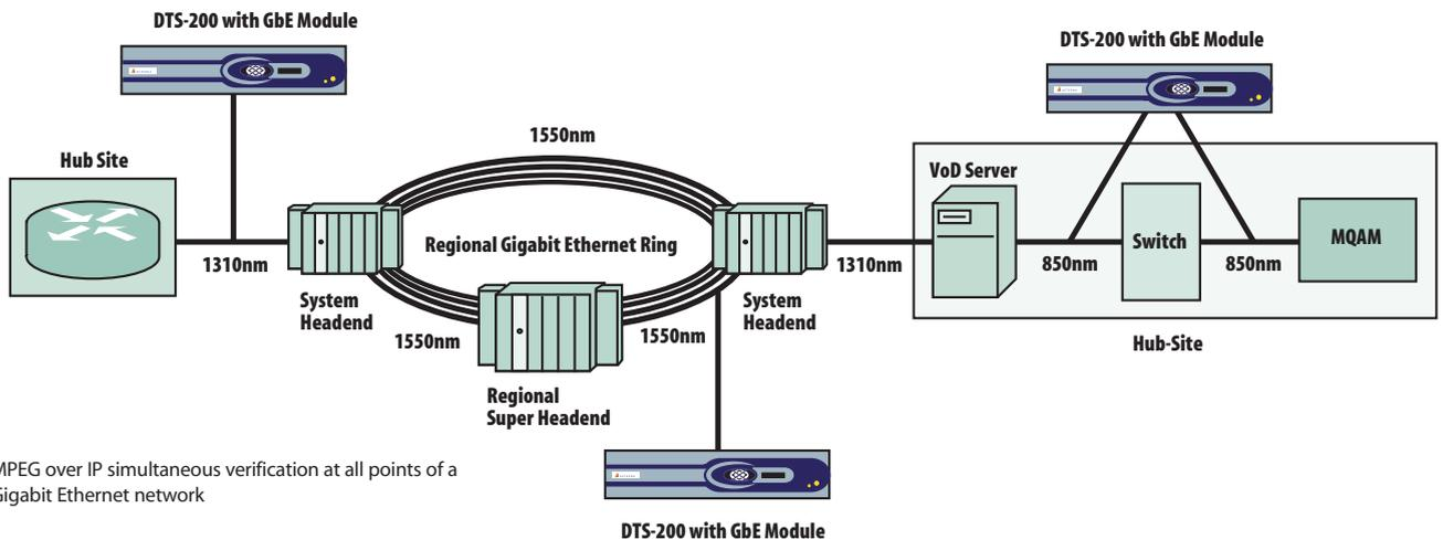
MPEG over IP simultaneous verification at all points of a Gigabit Ethernet network
