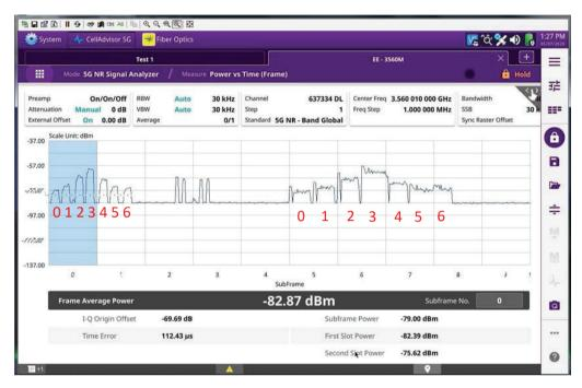
Figure 7. Above the 7 antenna array segments (marked in red) can be seen with their relative powers, antenna 3 is dominant
