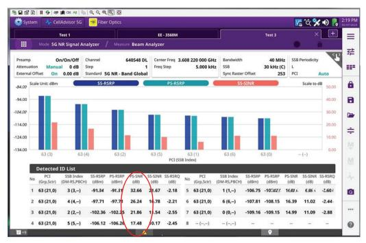
Figure 8. The CA5G Beam Analyzer '3' Network SCR Analysis
