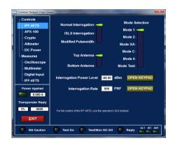
VirtualPanel software example for manual control of LRU
