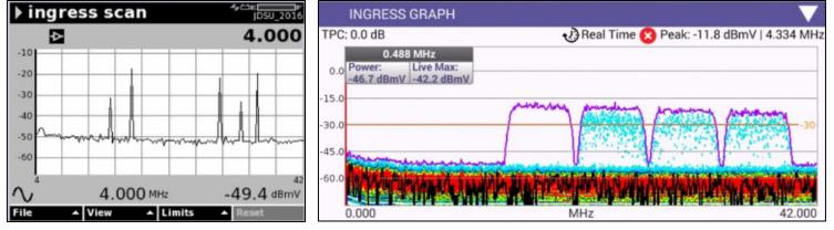
1 - Swept Spectrum Analyzer showing spikes where Cable modem traffic is present since it can only measure energy at frequencies it is currently turned to
