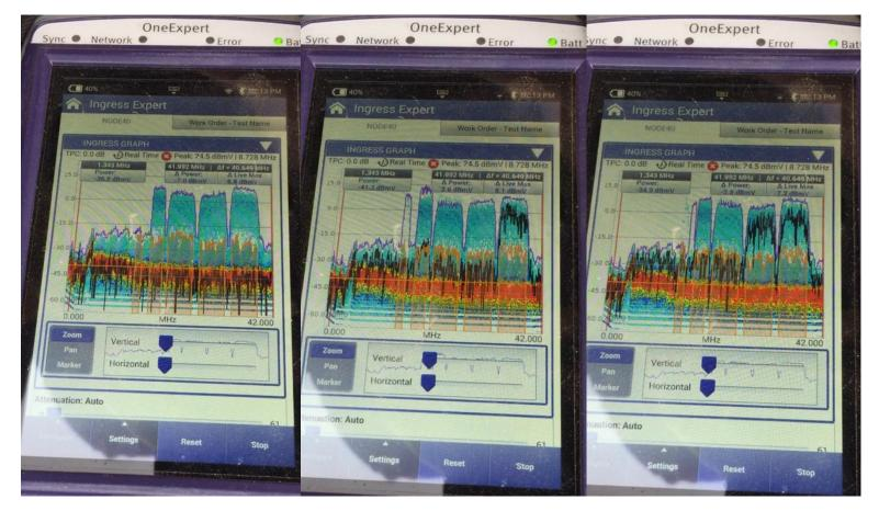
7. It was concluded the ONX was able to quickly detect the CPD on this node, however, due to time we were unable to track down the root cause of this particular issue.
