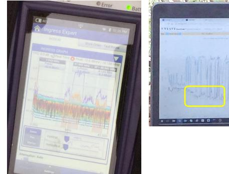
14. **Note on Traces:** During the investigation into this consistent noise source it appeared to be best visualized by activating the Live Max, Max Hold, and Heatmap traces. Other traces added little additional information while also cluttering up the screen, making it appear too busy.
