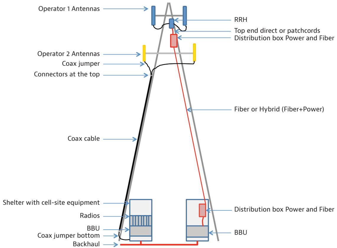
Figure 5: Common cell site structure and components
