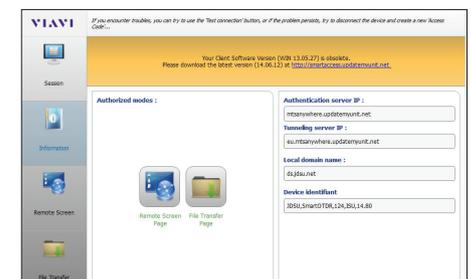
SmartAccess Anywhere, remote access and control of instrument for coaching and support of techs in the field, includes file transfer
