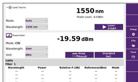
Built-in power meter and laser source
