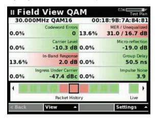
The Field View QAM dashboard shows a variety of measurements for the represented carrier, and indicates by color results outside of user-designated limits. From the dashboard the technician can select a measurement parameter to view more closely and switch directly to a full screen display of that measurement.
