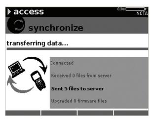
Users can synchronize test files from the field and administrators can update channel plans over Ethernet or DOCSIS RF connections.
