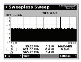
Sweepless Sweep provides a quick method to check cable system integrity using active channels to sweep the forward path. The method does not use inserted sweep points and no forward path headend gear is required.
