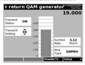
The ability to transmit a QAM-16 or -64 modulated signal back to the headend is helpful for proving line capabilities for future data and voice channels and for troubleshooting return path issues in the network.
