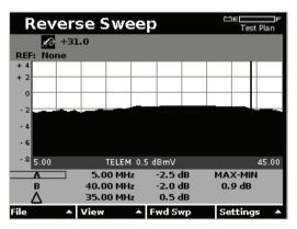
Tight reverse sweep points in the sweep plan display the entire return path with better resolution, and help to find mismatches or other problems in the upstream transmission path.
