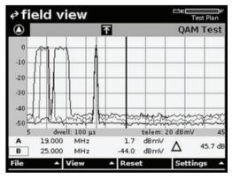
The optional Field View capability greatly improves the success rate and efficiency in locating return path ingress. Field technicians can view the return spectrum as received by the JDSU PathTrak Return Path Monitoring System. The DSAM allows for comparison of the remote spectrum with the local spectrum.
