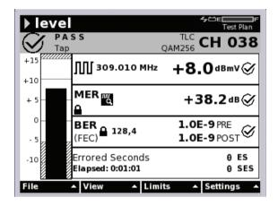
On a digital channel, the level mode measures the signal level and MER, and tracks the BER and errored seconds.
