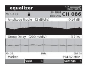
In-channel response and group-delay measurements help technicians troubleshoot narrowband RF transmission issues.
