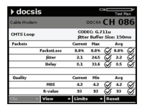
VolPCheck displays packet loss, jitter, and delay as well as MOS and R-values.
