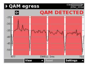
The QAM Egress option simplifies the detection of leaks (and verifying fixes) identified by leakage monitoring systems.
