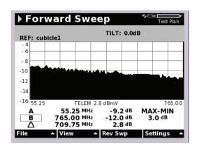
Forward sweep uses a unique referencing method to reveal accurately problems in the system without interfering with any of the analog or digital carriers.
