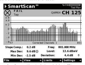
SmartScan provides a simple view to help locate RF issues between the tap and CPE.
