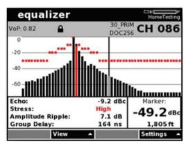
The equalizer tap graph shows reflections and the distance to the source.
