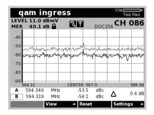
The QAM Ingress test lets technicians see spectrum underneath a live digital carrier which is usually not viewable due to the presence of the "haystack."
