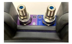
**WARNING:** Do NOT overtighten the F-81 adapter into the ONX's RF port, this can lead to permanently broken RF ports. Also, it is not recommended to use power tools when removing or replacing the F-81 adapters.
