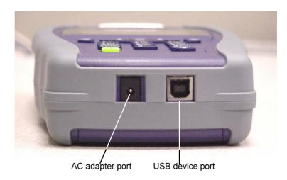
Figure 4 SmartClass bottom panel
