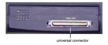
Figure 3 SmartClass E1 Tester right side panel
