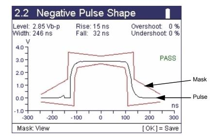
Figure 10 Pulse shape graph with mask
