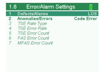
Figure 7 SmartClass E1 Tester Error/Alarm Settings menu screen
