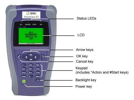
Figure 1 SmartClass front panel
