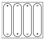
Figure 12 Battery orientation
