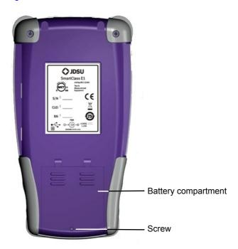
Figure 11 Back of SmartClass
