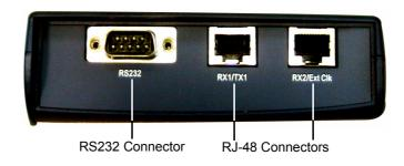
Figure 2 SmartClass E1 Tester left side panel
