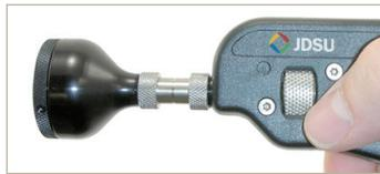
2. Align the adapter to the probe microscope and attach. Screw in to tighten and secure.
