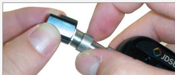
1. Align the notch-key configuration of **FBPT-COD** inspection tip to the probe microscope (with barrel assembly attached) and attach. Screw in to tighten and secure.
