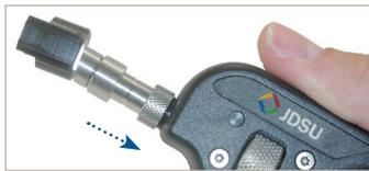
1. Align the notch-key configuration of **FBPT-COD-L** inspection tip to the probe microscope and attach. Screw in to tighten and secure.
