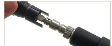
3. Attach the OptiTap plug to the CleanBlast system, apply light pressure to engage safety switch and initiate cleaning.
