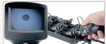
3. Apply light pressure to get optimal contact with the fiber end face, adjust focus, and inspect.
