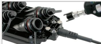
2. Align the **arc and flat** "male" pin geometry of the inspection tip to the matching "female" counterpart insertions inside the OptiTap receptacle adapter, insert to secure.
