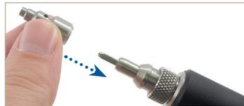
2. Align the cleaning mating adapter to the cleaning tip and secure.
