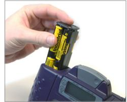
**Note:** NiMH rechargeable batteries cannot be recharged inside the HP2 display. They must be removed from the display unit and charged with a battery charger.
