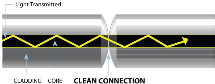
Today's connector design and production techniques have eliminated most of the challenges to achieving **core alignment** and **physical contact**. What remains challenging is maintaining a **pristine end face**.
