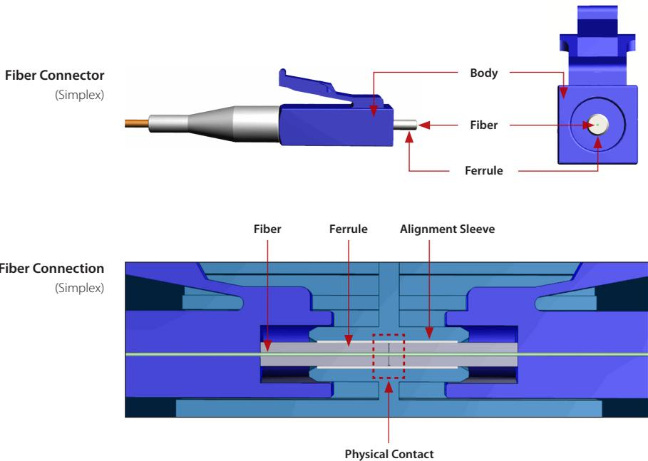
**Body** Houses the ferrule that secures the fiber in place; utilizes a latch and key mechanism that aligns the fiber and prevents the rotation of ferrules of two mated connectors.
