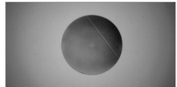
**Zones** **Zones** are a series of concentric circles that identify areas of interest on the connector end face. The inner-most zones are more sensitive to contamination than the outer zones.
