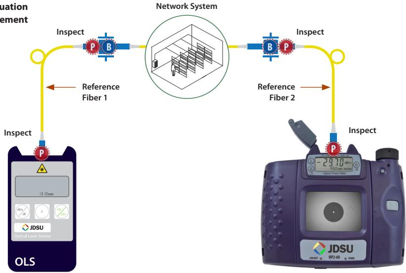
1. Disconnect the power meter from **reference fiber 1**.
