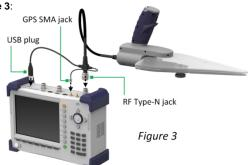
3 Initialize the connected handle to calibrate its built-in compass as described in the following section.
