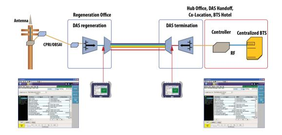
Figure 8. Testing xWDM-based fronthaul networks
