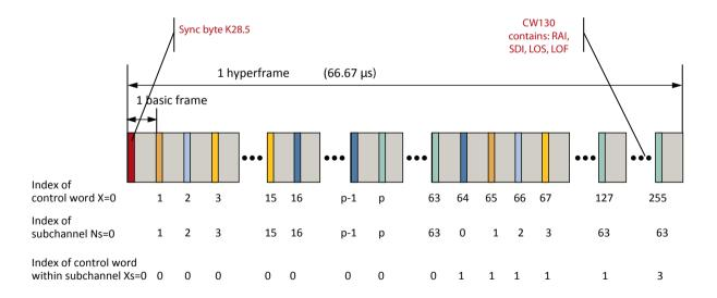
Figure 5. CPRI frame structure
