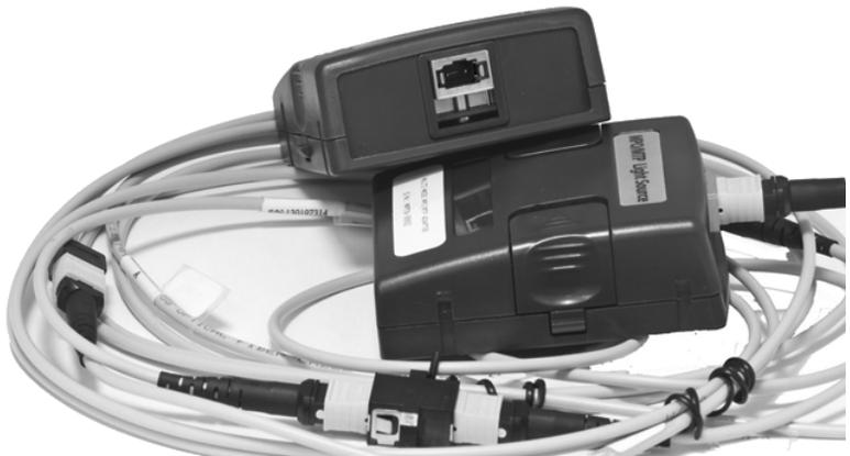
The purpose of this quick start guide is to provide the basic information required to use the JDSU NGC-4500 Multiple-Fiber Push-On/Pull-off (MPO) Multimode Fiber (MMF) Kit for the Certifier40G. Topics covered in this document include:
