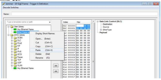
4) Now you have successfully move the frame from Trace View GUI to Maestro(Jammer) GUI used for Jamming. You can just click on the ">>" to move over that "Ether Frame-special iSCSI" as shown below to use as a Trigger or Jammed event.
