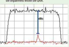
**Black is QAM Channel** Red is Noise below OAM Blue is difference between QAM carrier and ingress under the carrier (dBc)
