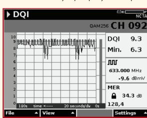
DQI makes troubleshooting intermittent QAM issues easier by simplifying results while at the same time increasing the sample rate of the QAM symbols
