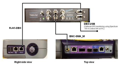
Figure 60 GPS Reference Timing Connection Diagram - 5800v1
