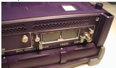
Figure 28 Fully inserted MSAM
