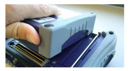
7 Seat the module into the connector with slight pressure.
