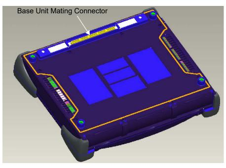
These connectors *must* be aligned carefully before connecting the module to the base unit.
