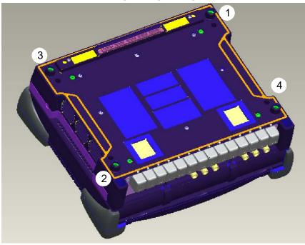
**Figure 25** Sequence for securing and tightening the screws
