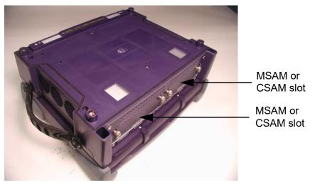
Figure 21 T-BERD/MTS 8000 base unit with a DMC
