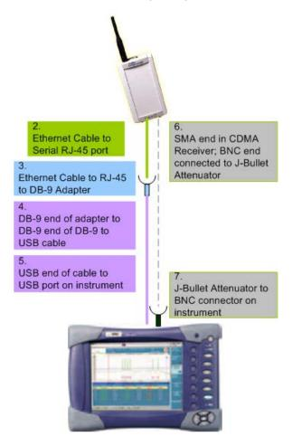
Figure 56 CDMA connection for one way delay measurements
