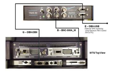
Figure 65 GPS Connection Diagram - MSAM v2 in MTS8000v2
