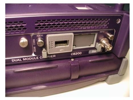
6 Push the PIM into the port until the PIM panel is flush with the exterior panel of the chassis, and the PIM ejection button pops out.
