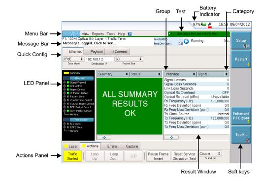
Figure 48 Main screen (Ethernet application)
