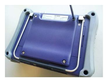
2 Remove the four screws that hold the back cover in place.
