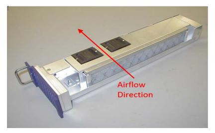
Figure 85 Fan tray assembly of MAP-2100, removed from the unit
