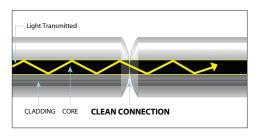
Today's connector design and production techniques have eliminated most of the challenges to achieving **CORE ALIGNMENT** and **PHYSICAL CONTACT.**
