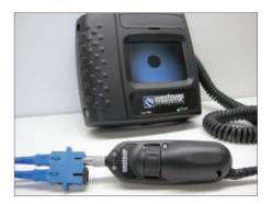
The FBE probe allows the inspection of "male" ends of fiber optic termination or installed fiber connectors quickly and easily. The practical use of the FBE probe eliminates the need to disassemble hardware devices prior to inspection while providing a clear image of the fiber end-face on the 3.5" LCD display.
