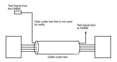
Fig. 1 Surveillance of a cable using a free fiber (or dark fiber)
