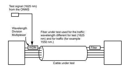
Fig. 2 Monitoring an active fiber (in service)
