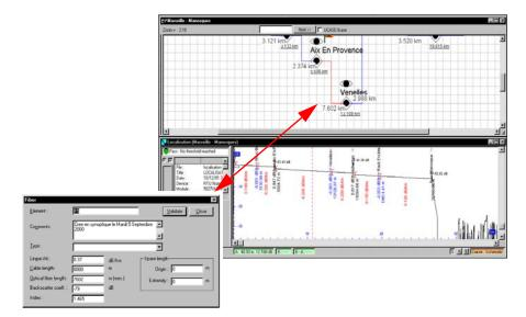
This readjustment allows the optical elements of a link to be localized precisely. When a fault is detected, the system can determine the intervention location, from a geographic position, due to the fact that it knows the optical and physical lengths of the fibers and cables.
