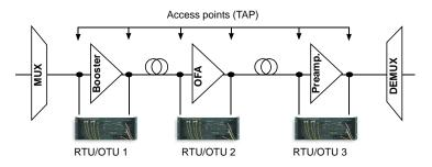
Fig. 110 Example of network with equipment (MUX, DEMUX, Amp, etc.) and monitoring RTUs connected to TAPs.
