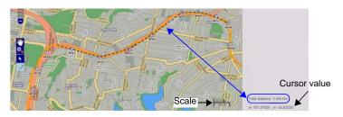
Fig. 194 Measuring a distance on the map
