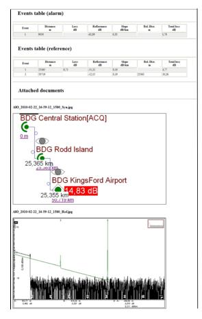
Fig. 143 Example of alarm report (OTDR)- part 3
