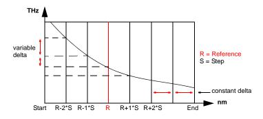
Fig. 126 Exemple with Step Unit = nm
