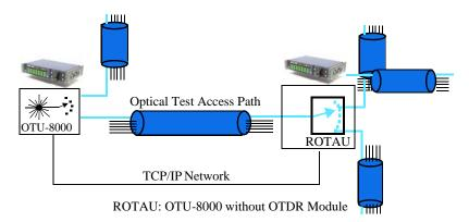
Fig. 51 Description Remote Optical Switch
