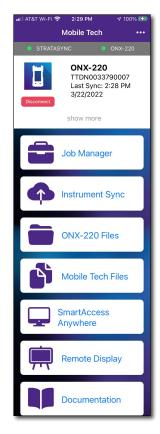
Job Manager – Attach jobs to tests, including customer info and work orders, and track test results
