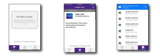
• **ONX-220 Files and Mobile Tech Files** – Manage files on the unit that you can save to your phone or tablet. Use the **ONX-220 Files** menu to manage files stored on your meter, use the **Mobile Tech Files** menu to manage those stored on your mobile device.
