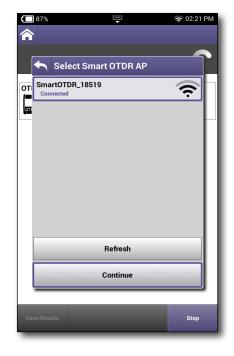
5. Once connected, set the fiber parameters. These settings will be saved for your next test.
