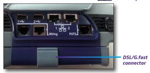
There are also two home wiring ports, one RJ11, one RJ45, one RJ11 POTS connector, and one RJ45 DSL connector (under the flap on the bottom module).
